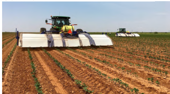
Blue River Technology's "see and spray" tech at work on a crop sprayer. | Image: Blue River Technology
