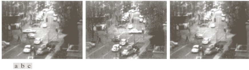
FIGURE 10.60 Building a static reference image. (a) and (b) Two frames in a sequence. (c) Eastbound automobile subtracted from (a) and the background restored from the corresponding area in (b). (Jain and Jain.)
