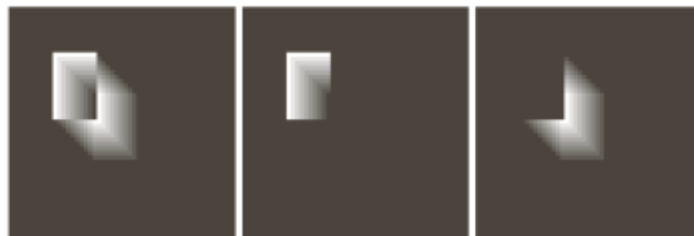
FIGURE 10.59 ADIs of a rectangular object moving in a southeasterly direction. (a) Absolute ADI. (b) Positive ADI. (c) Negative ADI.
