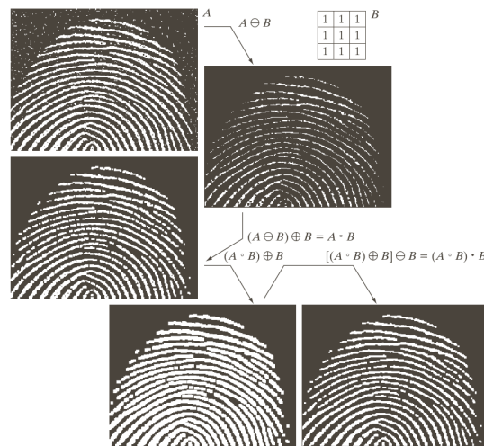
FIGURE 9.11 (a) Noisy image. (b) Structuring element. (c) Eroded image. (d) Opening of A . (e) Dilated opening. (f) Closing of the opening. (Original image courtesy of the National Institute of Standards and Technology.)
