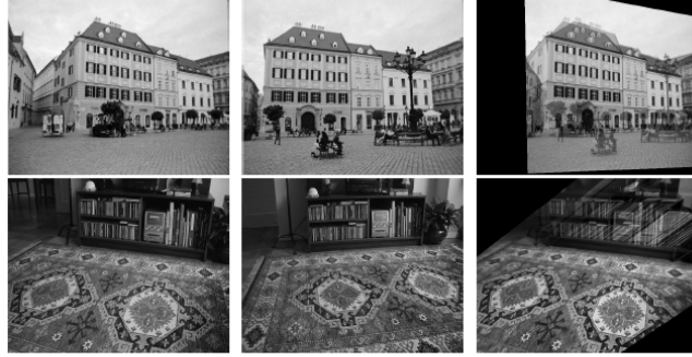
Figure 5.13. Homography between the left and middle images is determined by the building facade on the top, and the ground plane on the bottom. The right image is the warped image overlaid on the first image based on estimated homography H . Note that all points on the reference plane are perfectly aligned, whereas points outside the reference plane are offset by an amount that is proportional to their distance from the reference plane.
